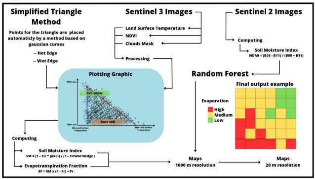
Figure 2-2: Diagram of the WaSCIA Soil Moisture and Evaporative Water Loss workflow.
