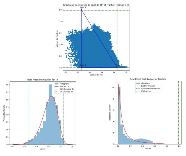
Figure 2-3: Simple Triangle approach used in this project.
